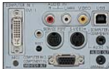
PLC-XU55/XU50 Terminal Input Panel
