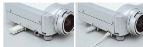
Wireless Networking with USB Wireless LAN Adapter (Left Image)
